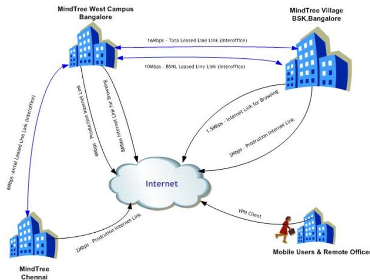
In engagements that need connectivity between the clients' and our network, connectivity is achieved through a dedicated communication link or a site-to-site VPN tunnel using our ODC model. The overall diagram showing the ODC setup is shown below.
