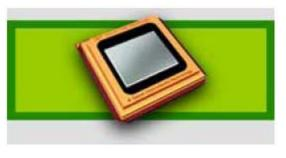
one pixel in a projected image. When a DMD chip is coordinated with a digital video or graphic signal, a light source, and a projection lens, its mirrors can reflect an all-digital image onto a screen or other surface. The DMD and the sophisticated electronics that surround it are what we call Digital Light Processing technology.
