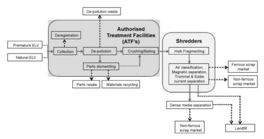
The ELV value chain supports a highly materially efficient trade loop between manufacturers and consumers, channeling valuable resources back into the manufacturing systems once their value as products, or as parts, is fully exhausted – but long after they entered the consumer market as new vehicles.
