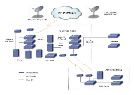
UTP - Unshielded Untwisted Pair - Multiple Means 2 Networks Connect on LAN
