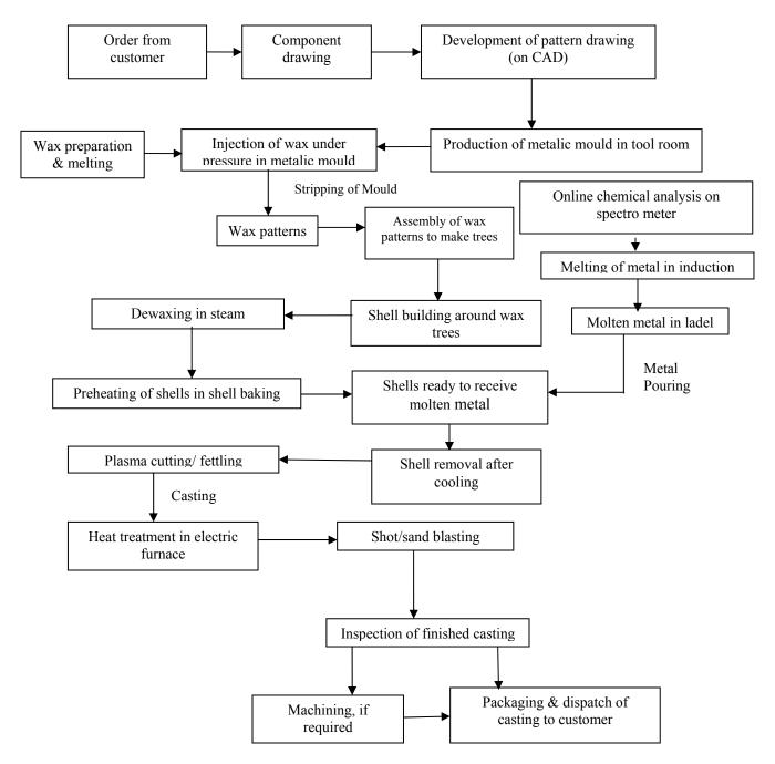
The production floor has a tool room with CAD / CAM engineering facility, machine shop, machinery for wax injection, shell production in temperature & humidity controlled environment, induction-melting furnaces, shot & sand blasting machines, Air plasma cutting machines, TIG welding machines, heat treatment furnace in addition to CNC & the conventional machining facility
