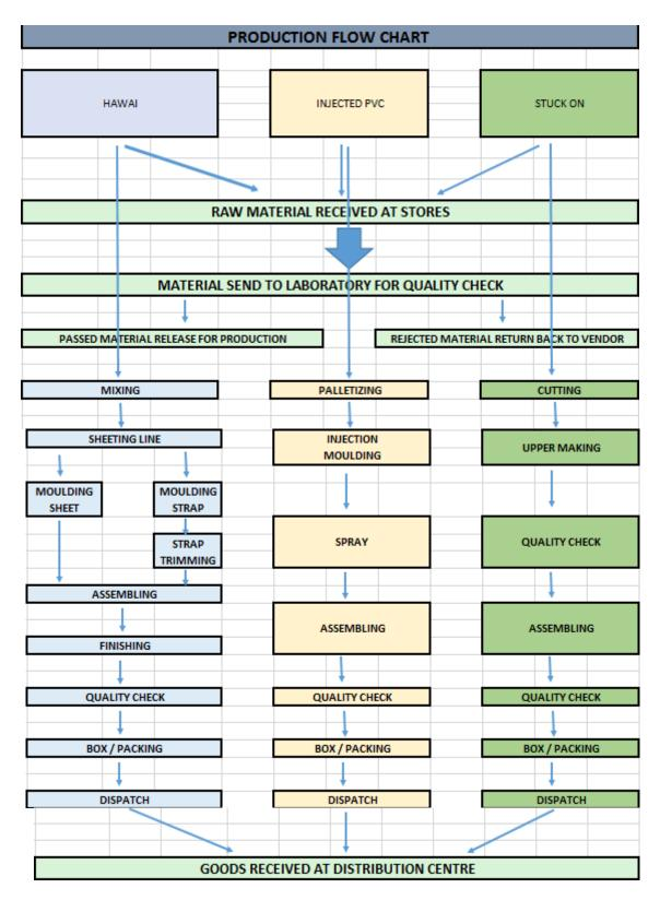
The manufacturing process can be broadly divided into five stages being, (i) mixing of compound; (ii) sheeting and palletizing; (iii) compressed and injection moulding; (iv) assembling; and (v) finishing and packing.
