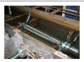
All flexible hoses and expansion joints are leak tested.
