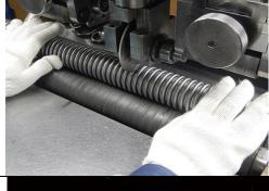
Flexible hoses are cut to the specified length as specified by the Customer's Specifications
