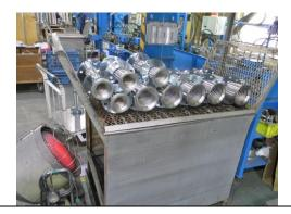
Water or other liquids must not remain inside products. Products are dried by warming them to evaporate remaining moisture, or pumping warm air into the product.
