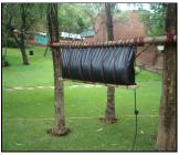
The Company has also developed manual pumps (peddle operated) that would not need power and a flexible storage tank. As per the system design, the farmer will collect the rain water through the field in the Poly lined ponds from where the water will be lifted using the manually operated pumps to a pedestal mounted storage tank for gravity flow irrigation.
