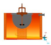
• The refining of lead is done through pyro-metallurgical process and removal of different elements is done by the addition of different reagents at required temperature with severe agitation to the lead bath.
