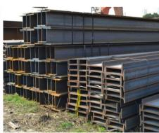
The Parallel Flange Beams come in different shapes depending upon the width & depth of the beam and are generally known as I-beam and H-beam. The H-beam has wider flanges than an I-beam, while the I-beam has tapered edges. Thus the main difference between both H-beams and I-beams is the flange by web ratio. The types beams further vary
