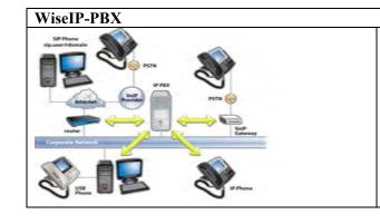
WiseIP-PBX is a Software based IPPBX platform that supports both TDM & IP technology (Interoperable Analog & Digital) that Supports all open source telephony hardware. Enterprise IP-PBX system is integrated with Unified messaging system such as SMS, Email, Video and Instant Messaging. Voice mail, Voice paging, Built-in IVR, personalized greetings, traditional calling, FAX and many more.
