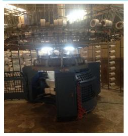
We have 25 machines used for Interlock, Rib, Fleece, Reversible and Polyfill knitting while 2 machines for manufacturing Sinker. We manufacture fabric using yarns varying in mixture of cotton, polyester and from count varying from 30 to 50 counts. Knitting machine used for Sinker is of 32 guage, 28 guage and 24 guage. It uses 102 yarns at a single point of time. Knitting machine used for other knitting varies from 13 inches to 34 inches in diameter.
