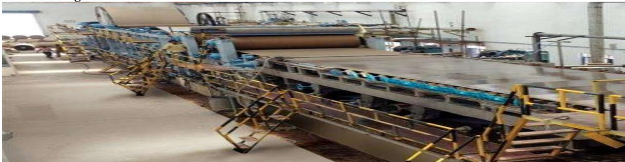
Corrugating roller is located at the base level and A liner is passed through pressurized rollers via dry steam another liner is passed through corrugated roller which gives the shape of corrugation to the middle liner and thus, corrugated waves are produced. 5 ply online corrugation machine with double profile flute for the combination of B and C flute carton which is as per the international norms and standards is used for the same. There are different hot plates and the adhesive for
