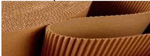
Kraft paper reels is placed on the corrugated machine. Corrugated waves are produced through steam which is generated through boiler plant.
