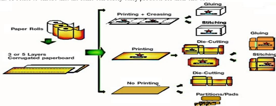
Printing is performed on corrugated box blanks that have been formed, scored and cut by a corrugator. The box blanks are subsequently cut or Die-cut into specific shapes for further forming into finished boxes. Printing Machine requires 2 main operators and 6 helpers in order to match the speed of the production.
