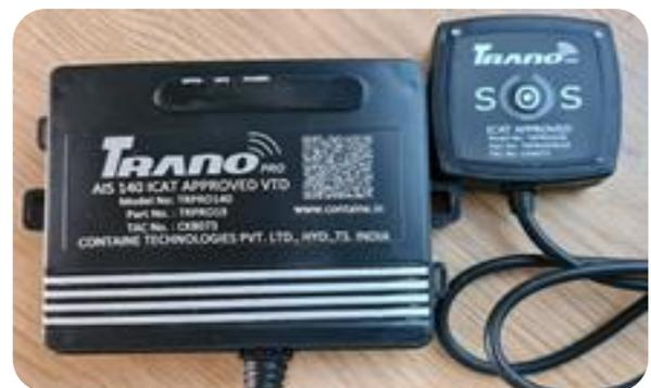
We have Tested AIS-140 (IRNSS) Vehicle Location Tracking Device in the Brand Name of TRANOPRO (TRPRO140) with SOS PANIC Switch (TRPROSOS) from ICAT -IMT - Manesar, Gurugram, Haryana State, vide: TAC NO.CK8073 (Certificate No. CT0GP8538) Dated: 27.06.2019, and Completed TWO COP’s.
