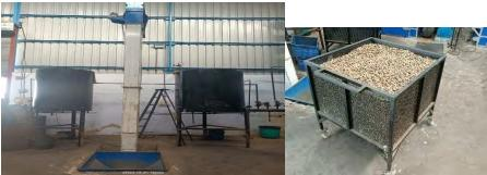
Once Raw Cashew Nuts are dust cleaned, it's getting load thru Elevator in Tank for steaming thru IBR. The process of steam boiling helps in soften the outer shell and removal of this shell with minimal effort. On completion of Boiling all nuts been offloaded in trolley and leave for cooling period.
