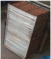
Separated Nuts collected from Scooping Line are filling in Tray and Trolley and loaded in Dryer to remove Oil from Husk of the cashew. Drying process vary between 350 Minutes to 480 Minutes depending on the Raw Material.
