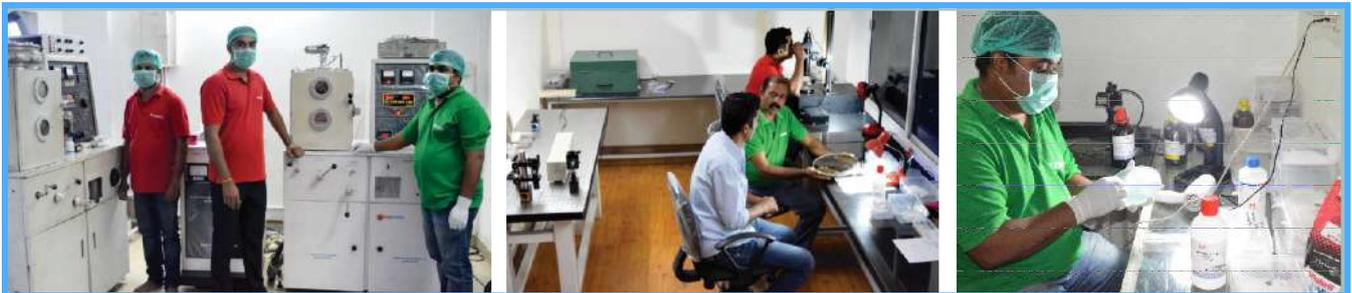
The Thin Film Coating Lab at Holmarc uses Vacuum coating chambers, Thin film reflectometer, Spectroscopic ellipsometer and spectrophotometers that aid in the creation of thin film optical coatings. A team of experienced engineers and technicians design, deposit, and measure thin film coatings ranging from our standard anti-reflective coatings to metallic mirror coatings.
