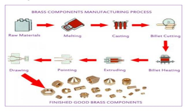
**Manufacturing of Brass Billets and Brass Rods**
